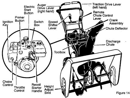
Auger Drive Lever – Starts and stops the auger and impeller (snow gathering and throwing)
